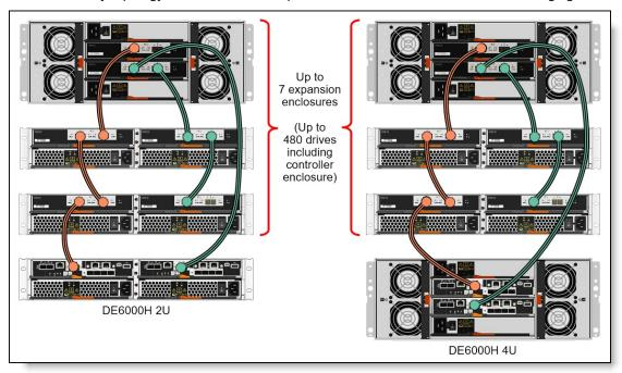
Figure 8. DE Series expansion enclosure connectivity topology
